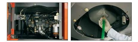
Wide doors give access, from ground level, to the fuel filter, water separator and engine oil filter. A large handrail, steps and anti-skid plates lead to the engine cover. The engine oil pan is fitted with a drain coupler. When draining, an associated drain hose is connected to the drain coupler. The drain coupler is reliable, avoiding oil leakage and vandalism.
