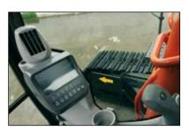
The colour LCD monitor, located in the cab, indicates coolant temperature, fuel level, and maintenance data. It also allows one-touch adjustment of the attachment. The display can also be adjusted to day or night shift.
