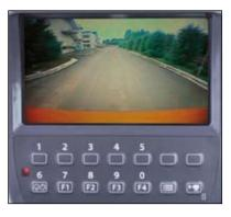
The widescreen colour LCD can also provide a view to the rear of the machine. Enhanced safety during swinging and travelling is the key advantage.
