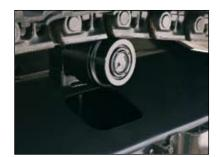
The X-beam is strengthened by the improved construction and enlarged box sections. The section is increased in strength up to 45%. Top and bottom plates of the X-beam use monolithic plates, instead of conventional welded four plates. This eliminates welding to strengthen the X-beam. Upper and lower rollers and upper roller brackets are increased in size for higher durability. Track links are thickened and reshaped for higher durability and rigidity.
