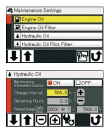
Replacement timing of hydraulic oil and fuel filters is alerted to the operator through the LCD monitor according to the schedule preset by the user each time when turning the key switch. The scheduled maintenance can prevent the failure of the machine. Attachement support system (work mode selector)
