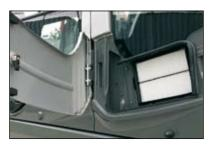
The fresh air filter for the air conditioner is relocated to cab door side from conventional location behind the operator seat. This allows easy cleaning and replacement of the fresh air filter, like the air circulation filter inside the cab.
